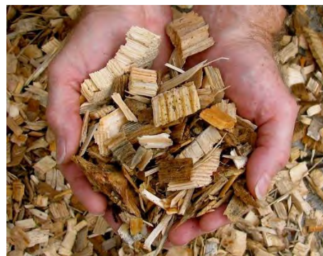
EXHIBIT 3-2: Example Wood Chips Used for Direct Combustion Plants
